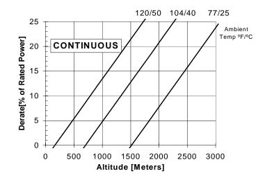
**NOTE:** Derates shown are based on 15 in H<sub>2</sub>0 air intake restriction and 2 in Hg exhaust back pressure.
