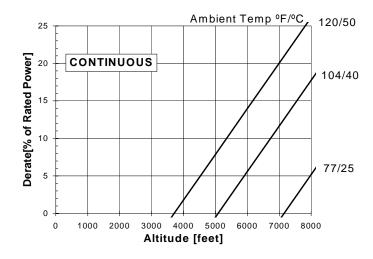
NOTE: Derates shown are based on 15 in H<sub>2</sub>0 air intake restriction and 2 in Hg exhaust back pressure.
