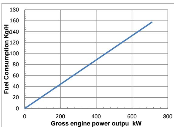
Curves shown above represent gross engine performance capabilities obtained and corrected in accordance with SAE J1995 conditions of 29.61 in. Hg(100kPa) barometric pressure [300ft.(91m) altitude] 77deg F (25 deg C) inlet temperature, and 0.30 in. Hg(1kPa) water vapor pressure with No.2 diesel fuel.
